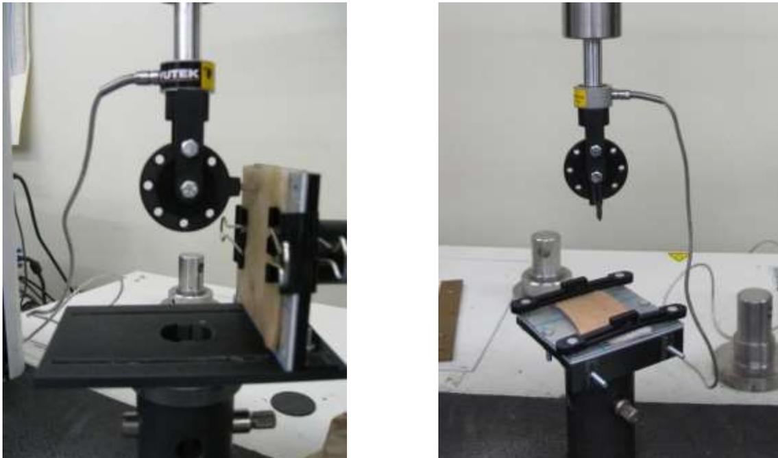
Figure 2.14: #15 Scalpel Slicing Test (left) #15 Scalpel Puncture Test (right)
