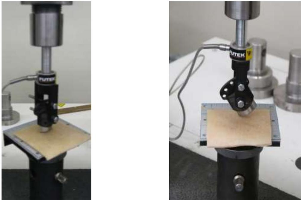
Figure 2.10: Vertical (90°) Puncture (left) Angled (56°) Puncture (right)
