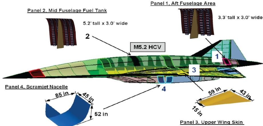
**Figure 1. Critical panels of the DARPA Falcon HTV-3X designed for Mach 5.2.**
