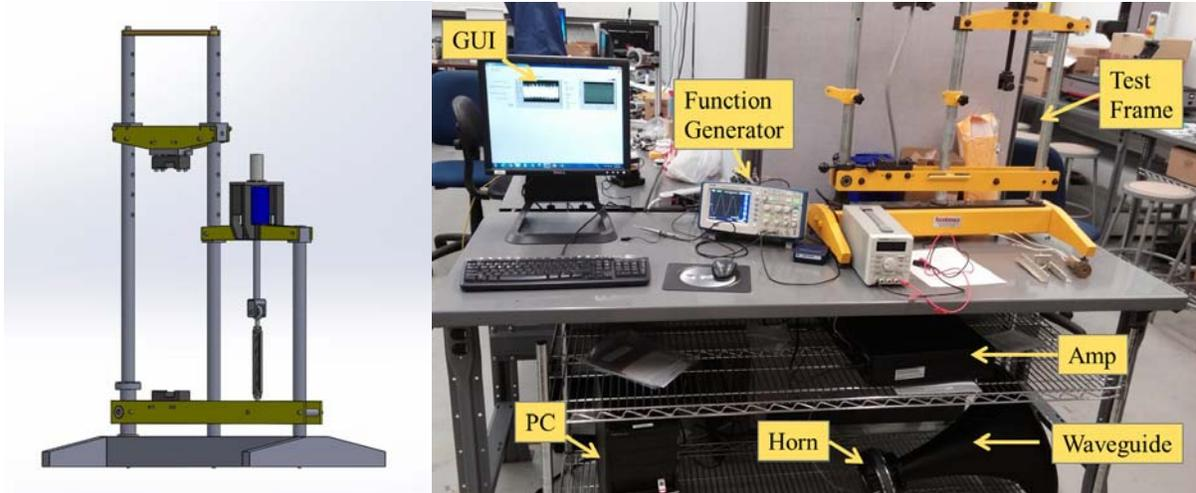
**Figure 2. (left) Numerical concept of column buckling frame and (right) physical test platform.**
