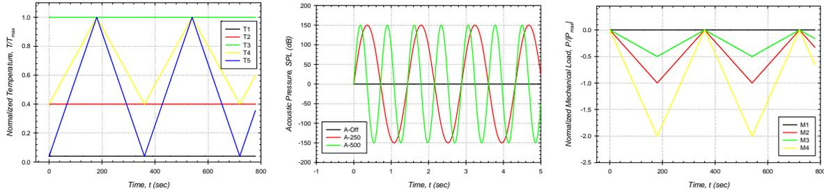
**Figure 3. (left) Temperature, (middle) acoustic, and (right) mechanical waveforms generated by the test device.**
