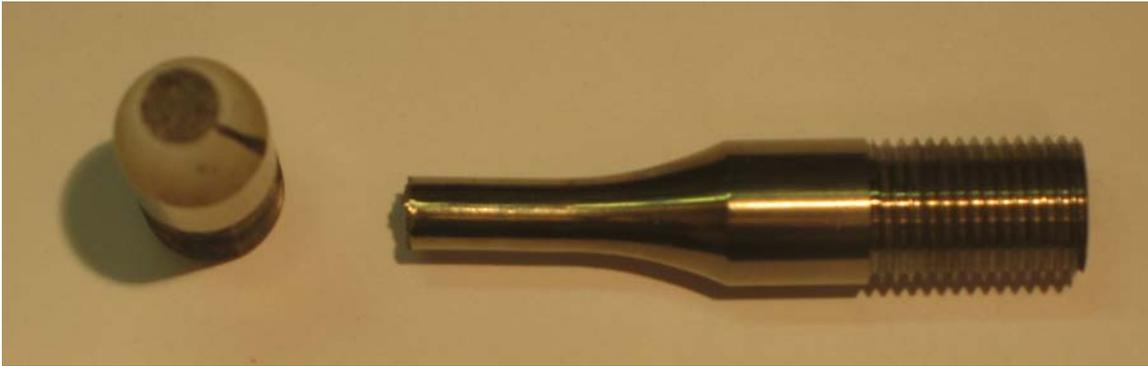
**Figure A.19. Photograph of fractured specimen D912-2, 400°C test temp and 1.5% strain range.**
