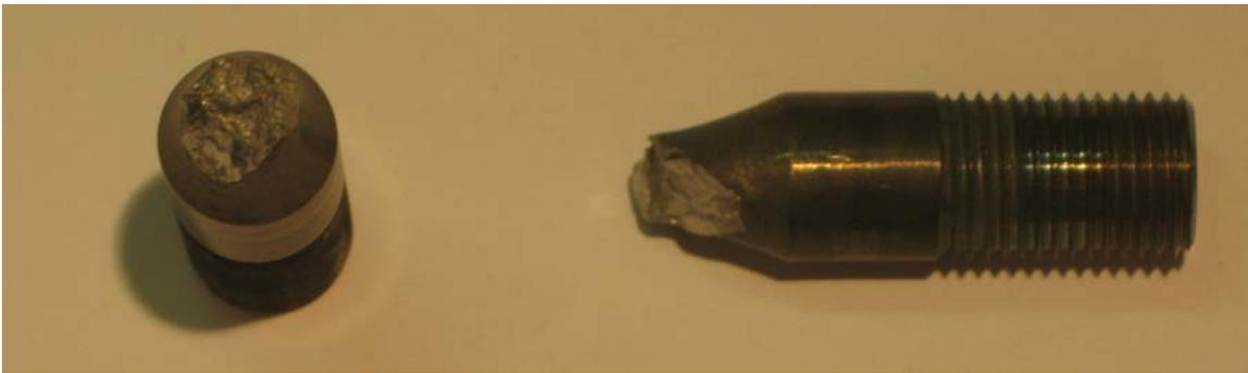
**Figure A.20. Photograph of fractured specimen D912-6, 750°C test temp and 1.2% strain range.**
