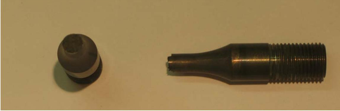
**Figure A.21. Photograph of fractured specimen D912-14, 750°C test temp and 1.4% strain range.**
