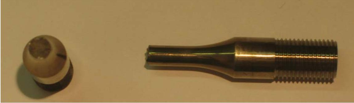
**Figure A.18. Photograph of fractured specimen D912-1, 400°C test temp and 1.5% strain range.**
