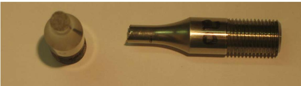
**Figure A.14. Photograph of fractured specimen D912-20, 24°C test temp and 1.2% strain range.**
