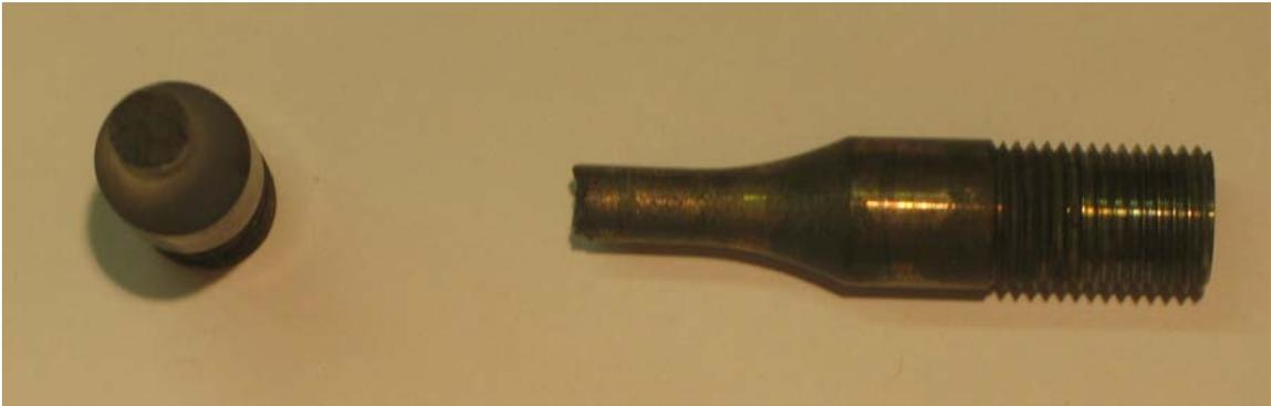
**Figure A.25. Photograph of fractured specimen D912-11, 850°C test temp and 1.6% strain range.**
