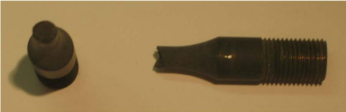
**Figure A.23. Photograph of fractured specimen D912-16, 850°C test temp and 1.2% strain range.**
