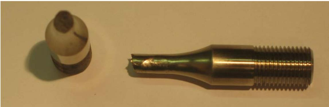
**Figure A.17. Photograph of fractured specimen D912-33, 400°C test temp and 1.2% strain range.**
