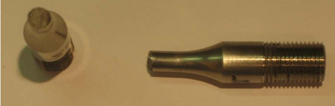
**Figure A.12. Photograph of fractured specimen D912-35, 24°C test temp and 0.8% strain range.**
