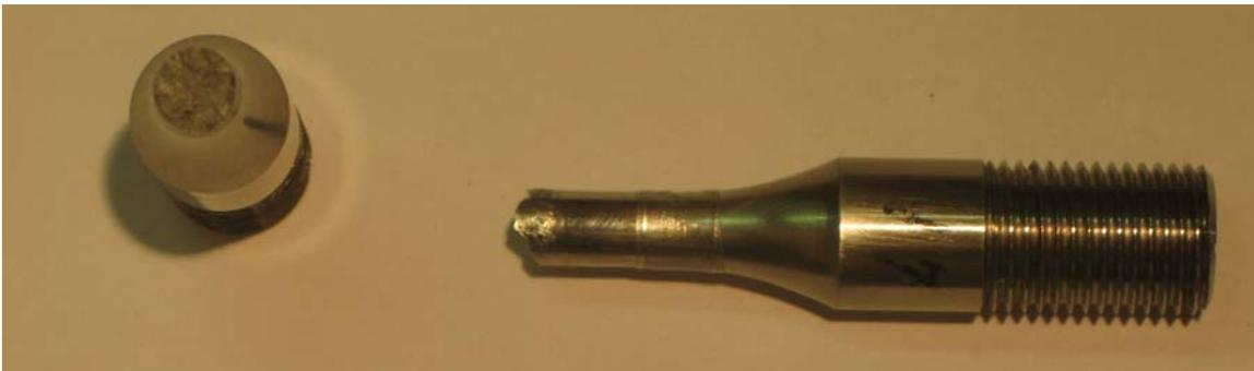
**Figure A.13. Photograph of fractured specimen D912-17, 24°C test temp and 1.0% strain range.**
