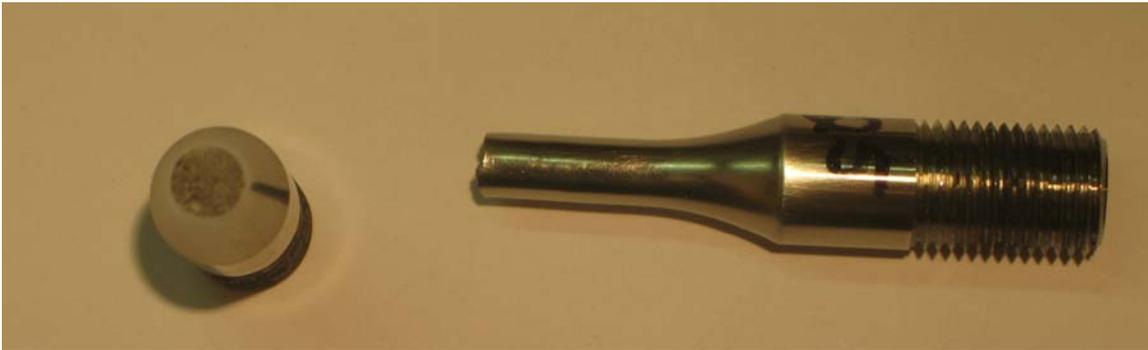
**Figure A.16. Photograph of fractured specimen D912-25, 24°C test temp and 1.6% strain range.**
