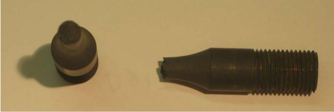
**Figure A.24. Photograph of fractured specimen D912-15, 850°C test temp and 1.4% strain range.**
