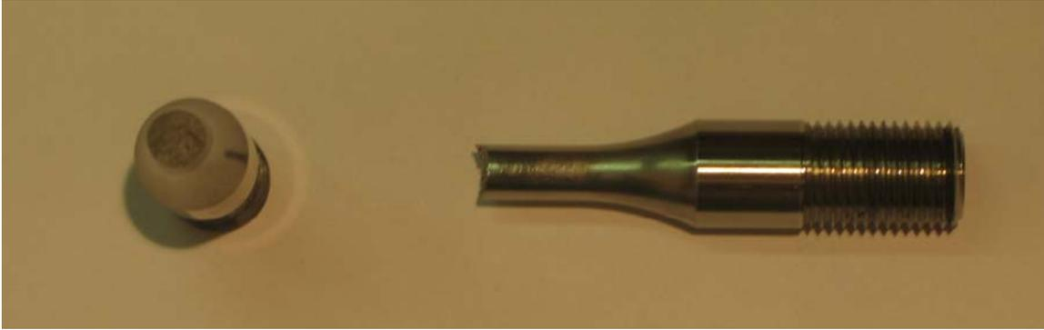
**Figure A.15. Photograph of fractured specimen D912-19, 24°C test temp and 1.4% strain range.**
