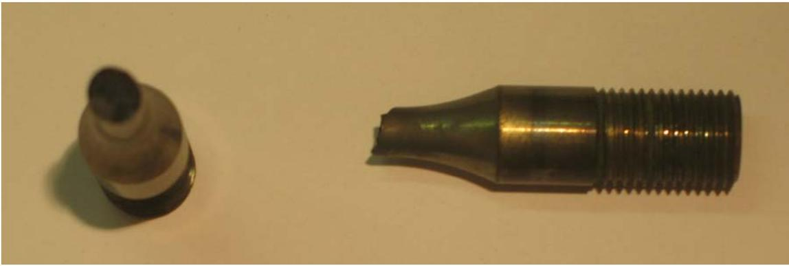
**Figure A.22. Photograph of fractured specimen D912-8, 750°C test temp and 1.6% strain range.**
