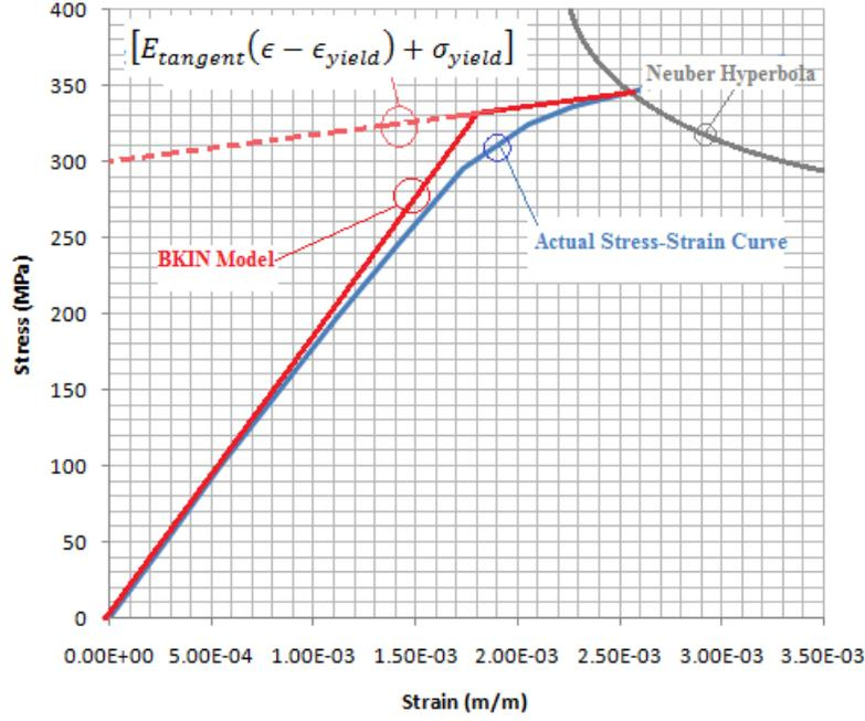
**Figure 11: BKIN model used to approximate the material behavior**
