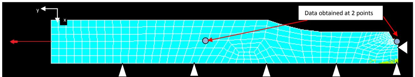
Figure 13 Specimen Constraints
