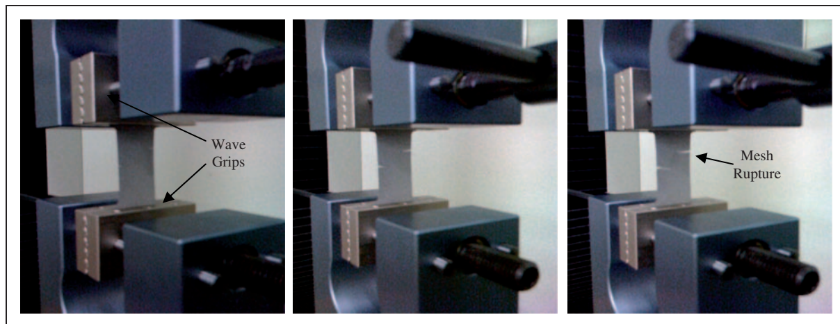
Figure 3. Time-lapse photography of CRE tensile test conducted on 316 L stainless steel 325 × 2300 mesh specimens in the warp (0°) orientation.
