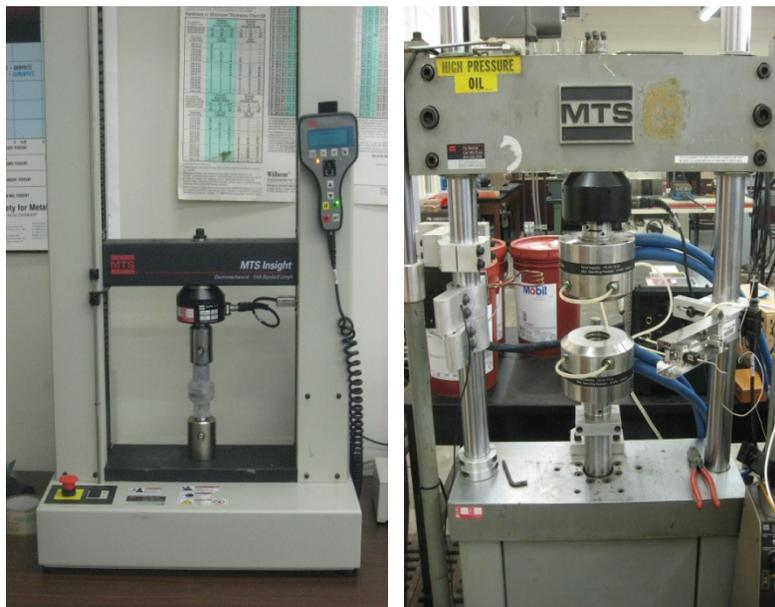
**Figure 3.1:** MTS Insight 5 (left) and Servohydraulic (right) load frames.
