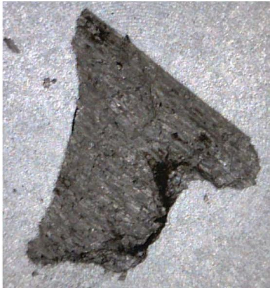
*Figure 4.18: Intergranular flake from specimen incubated in liquid Hg (S-L-30).*
