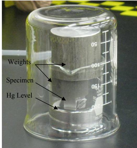
**Figure 3.18:** Pre-soaking of specimen in Hg prior to pre-cracking routines.
