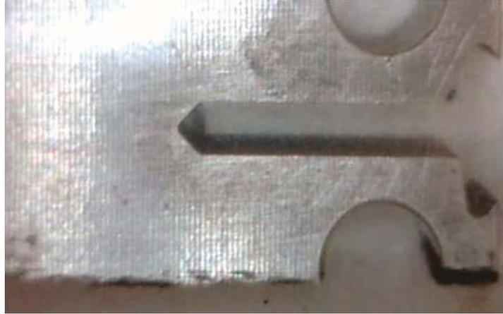
**Figure 3.23:** Failure of specimen through load pin hole.
