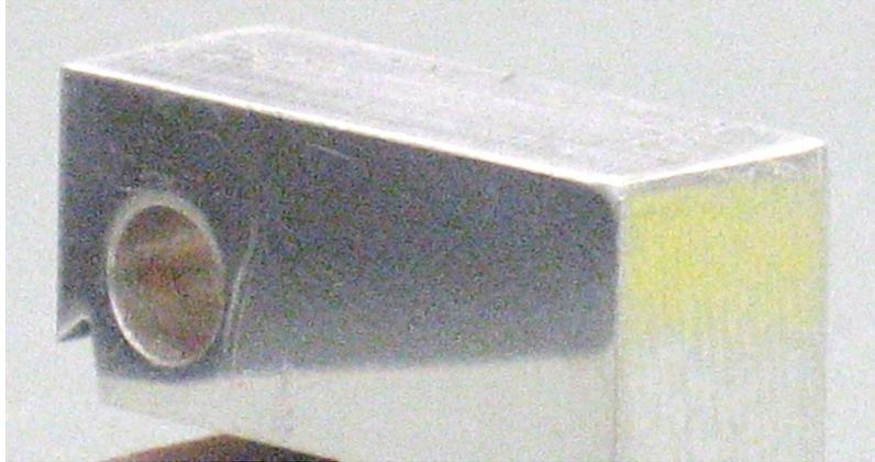
*Figure 3.12: Specimen surface after sanding and polishing with 1  $\mu\text{m}$  alumina powder.*
