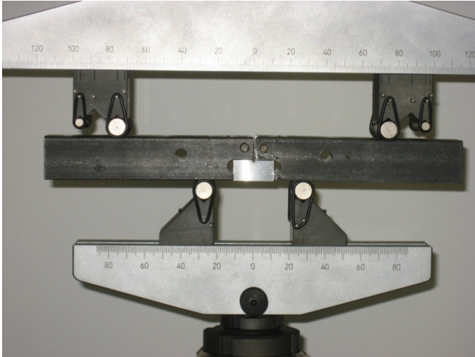
Figure 5: Rigid arms attached to C(T) specimen to be used in four point bending.
