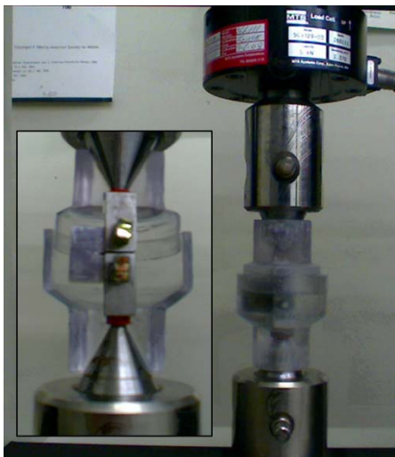
Figure 1: Environmental chamber shown attached to the MTS Electromechanical Tensile Load Frame, along with cutaway view including specimen.
