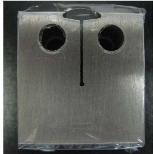
**Figure 3:** Blunt notch specimen with sleeve used in containing liquid at the notch/crack tip.
