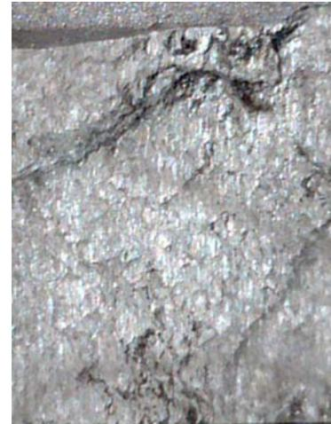
**Figure 6:** Fracture surface of specimen fractured in mercury with extensive cracking and burn markings (S-L-10).
