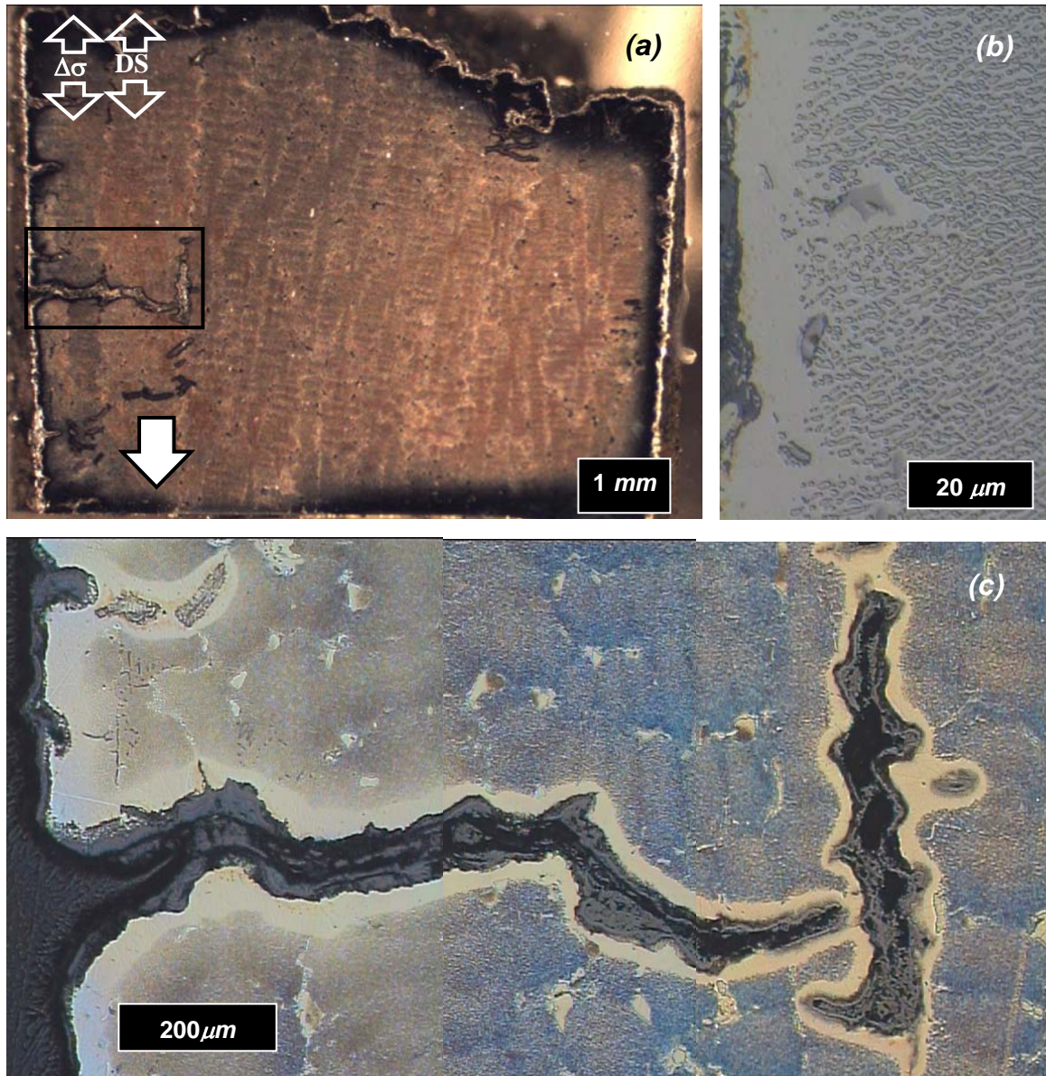
Figure 4.31: Crack initiation of creep-fatigue tested L-oriented DS GTD-111 under \dot{\epsilon} = 0.5\%/s , R_{\dot{\epsilon}} = -1 , \Delta\epsilon = 1.0\% and T = 1038^\circ\text{C} . For this case t_h = 10 min in tension.
