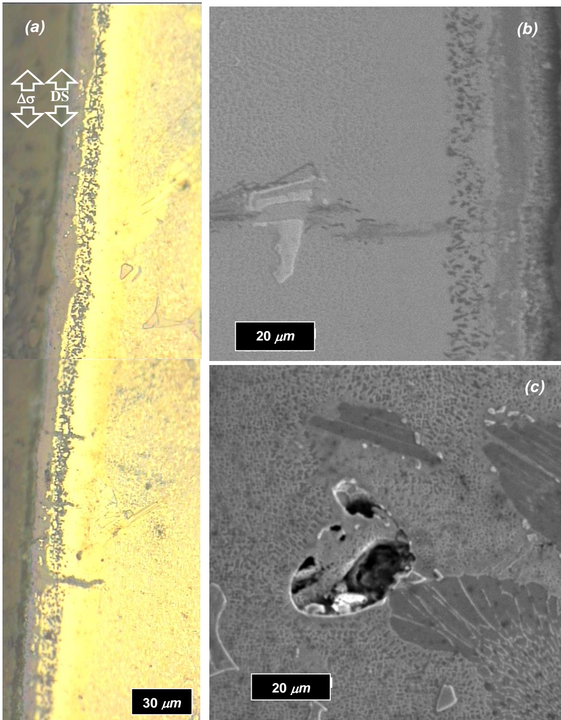
Figure 4.26: Crack initiation of creep-fatigue tested L-oriented DS GTD-111 under \dot{\epsilon} = 0.5\%/s , R_{\epsilon} = -1 , \Delta\epsilon = 2.0\% and T = 871\text{ }^{\circ}\text{C} . For this case t_h = 2\text{ min} in compression (Specimen ID: GTD-HC10 (L)).
