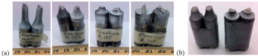
Figure 4: (a) The specimens were spray painted in black and white before the ELCF test for optical measurement and digital imaging correlation. From left to right are R0, R1, R2, and PE, respectively. (b) Fractured specimens after ELCF tests of R1( a/R=1/3 , left) and R2( a/R=1 , right)
